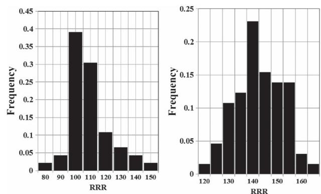
Fig. 5. The histograms of RRR values for Nb<sub>3</sub>Sn strands heat treated by Cycle A (Samples-6) and Cycle B (Samples 7).
