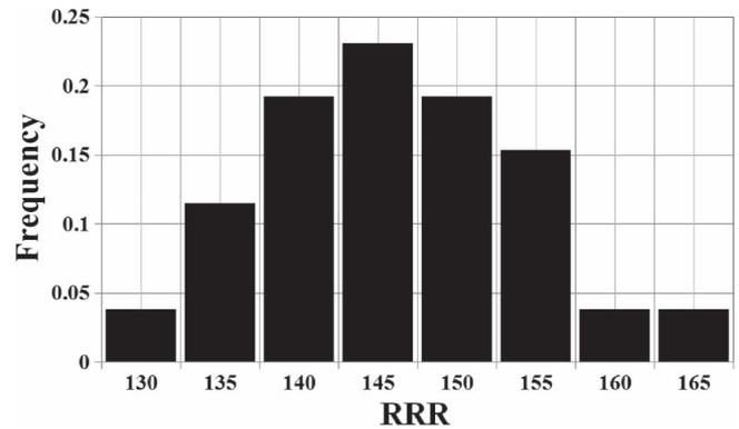
Fig. 4. The histogram of RRR values of Nb<sub>3</sub>Sn strands taken from compacted TF conductor sample in the course of Destructive Examination (Sample-5).
