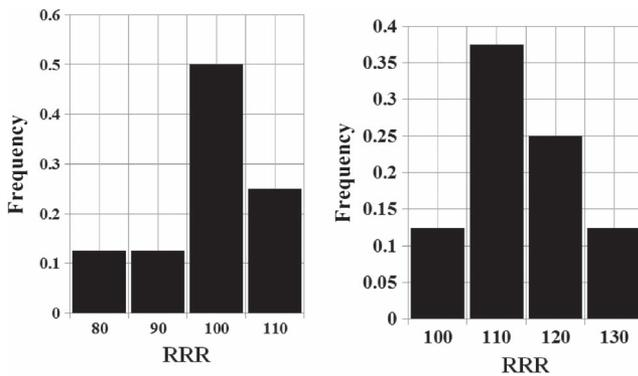
Fig. 7. The histograms of RRR values for Nb<sub>3</sub>Sn strands taken from high field zone (Sample-9—near spiral, Sample-10—near jacket).
