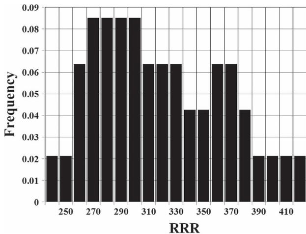
Fig. 2. The histogram of RRR values in certificates of Nb<sub>3</sub>Sn strands (Sample-1).
