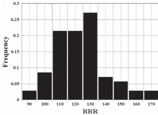
Fig. 6. The histogram of RRR values for Nb<sub>3</sub>Sn strands taken from low field zone (Sample-8).
