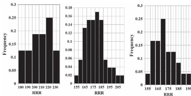
Fig. 3. The histograms of RRR values of Nb<sub>3</sub>Sn strands before and after electrochemical cleaning and Cr-plating (Samples-2,3,4).
