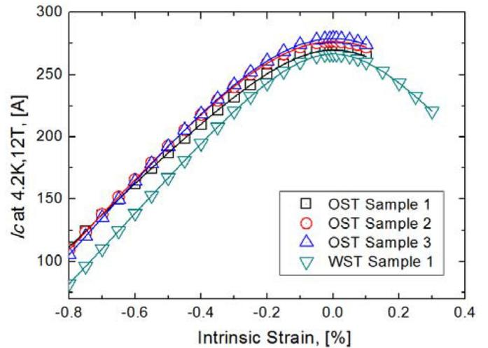
Fig. 3.  $I_c$  values as a function of intrinsic strain for the CNDA Nb<sub>3</sub>Sn TF strands.
