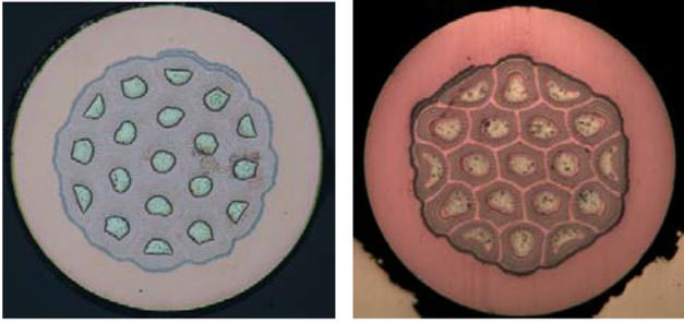
Fig. 1. Transverse cross-section of ITER TF Nb<sub>3</sub>Sn strands made by OST (left) and WST (right).
