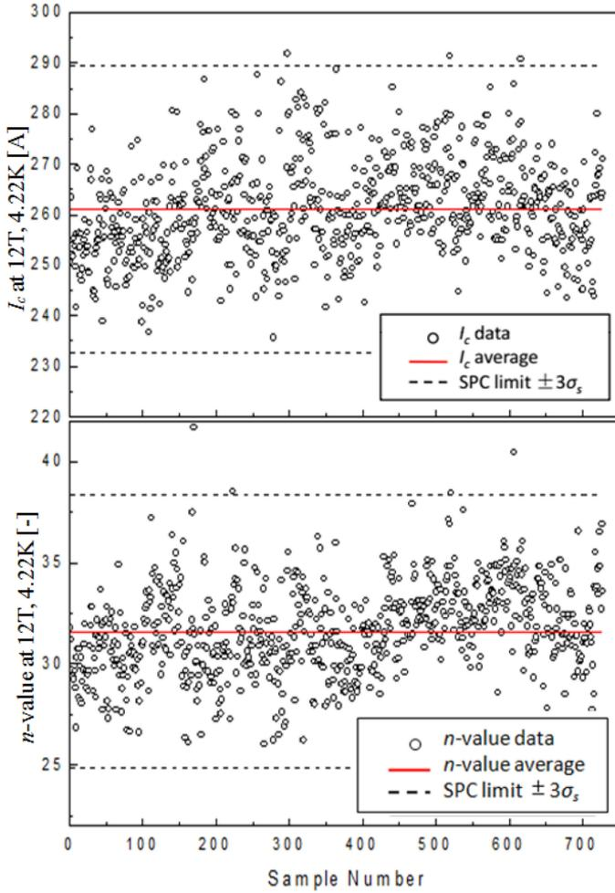
Fig. 2.  $I_c$  and  $n$ -value distribution in the TF WST Nb<sub>3</sub>Sn strands from the verification results.
