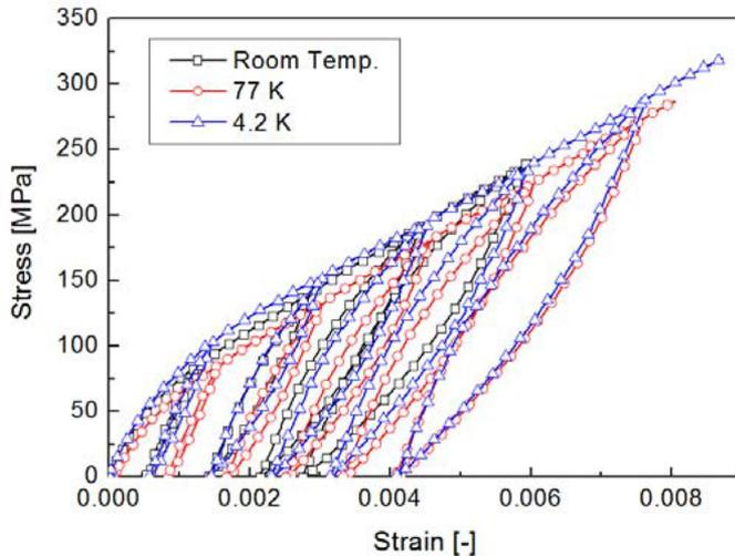
Fig. 4. Typical stress-strain curves for WST Nb<sub>3</sub>Sn TF strands.
