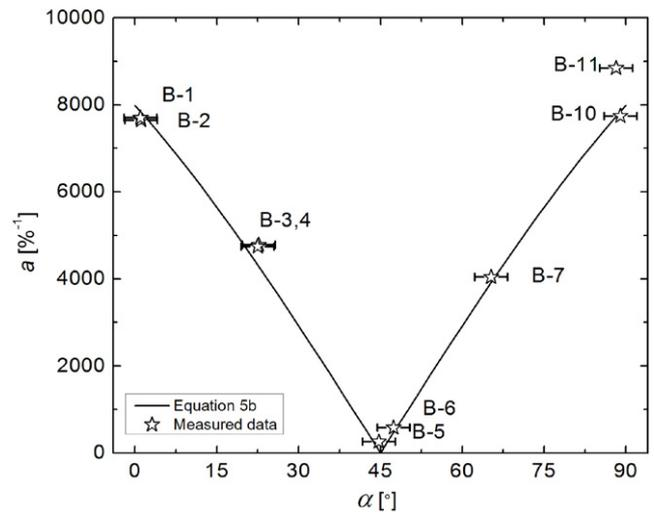
**Figure 7.** The strain sensitivity parameter  $a(\alpha)$  is plotted as a function of angle  $\alpha$  between the applied strain and the [100] and [010] directions of the superconducting film. The error bars of  $\pm 2.5^\circ$  include the uncertainty in the orientation of the patterned bridges with the conductor axis and the uncertainty in alignment between the applied strain and the bridge. The solid line is the expected angular dependence of  $a(\alpha)$ , expressed by equation (5b).
