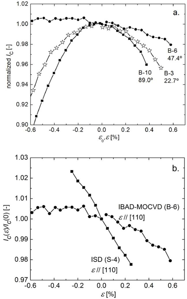
**Figure 6.** (a) Normalized  $I_c$  as a function of intrinsic strain  $\varepsilon_0$  of samples B-3 and B-10 and as a function of applied strain for sample B-6 at 76 K, highlighting the change in strain sensitivity with in-plane strain orientation. The solid lines are a fit to the data with equation (1). (b) Comparison between the strain dependence of the normalized  $I_c$  of IBAD-MOCVD sample B-6 and ISD sample S-4 at 76 K.
