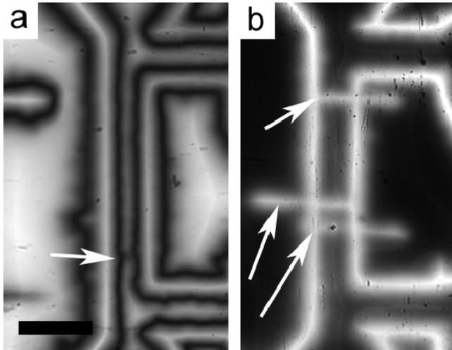
**Figure 2.** (a) Magneto-optical image of sample B-11 taken after the sample was field-cooled to 7 K in a field of 120 mT. The image shows a small defect, indicated by the arrow, running across the bridge width. (b) Magneto-optical image of sample B-12 taken at 60 mT, after the sample was cooled in zero field to 7 K, showing easy magnetic flux penetration along three large defects running across the bridge width, indicated by the arrows. The scale bar on the left is 300  $\mu\text{m}$ .
