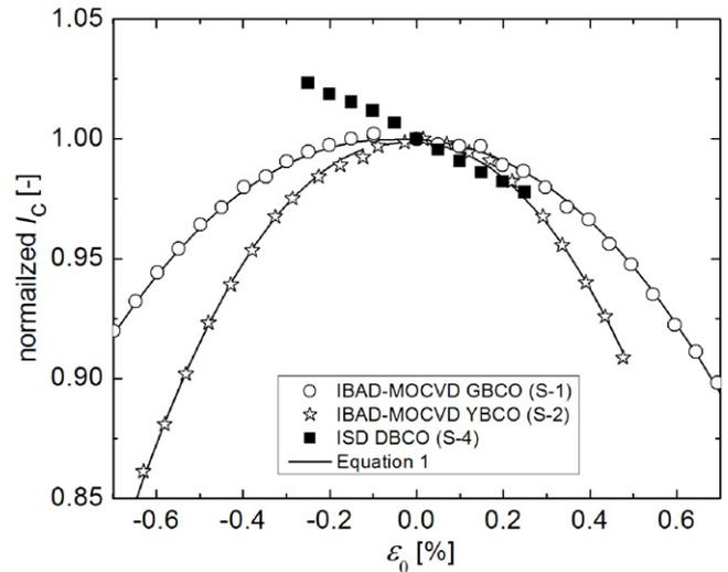
**Figure 3.** Normalized critical current as a function of intrinsic strain at 76 K for IBAD-MOCVD GBCO sample S-1, IBAD-MOCVD YBCO sample S-2, and as a function of applied strain for ISD DBCO sample S-4. The data shown are fully reversible. The solid lines are fits to the data according to equation (1).
