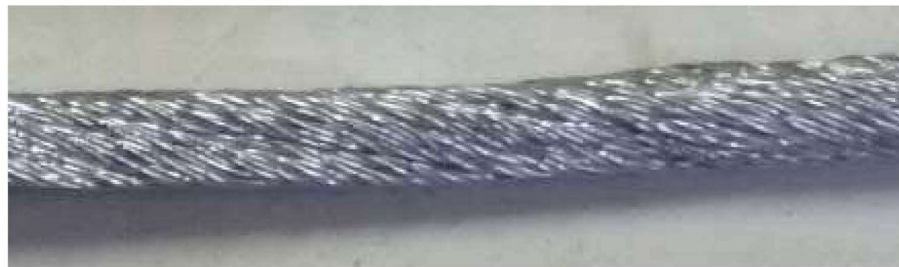
(c) CS conductor (short twist pitch)
