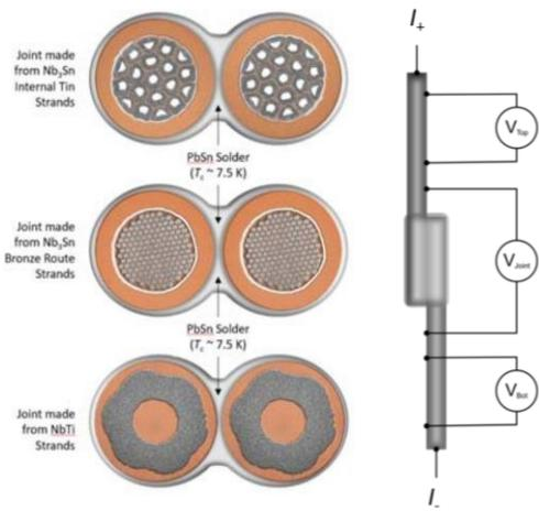
Below 7.5 K the joint solder superconducts and ceases to contribute to joint resistance. At that point the resistance is due to strand architecture
