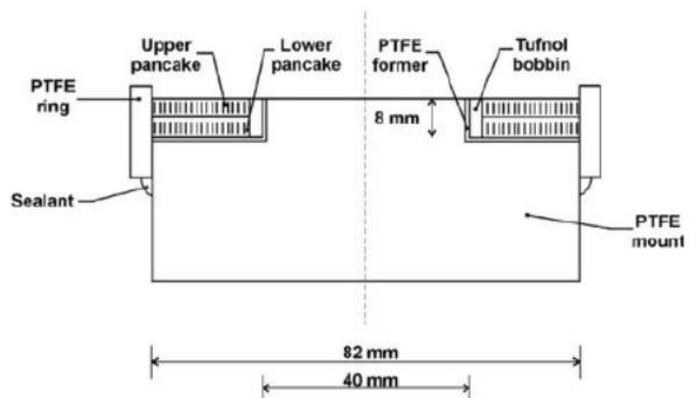
PTFE components used during the vacuum resin impregnation process.
