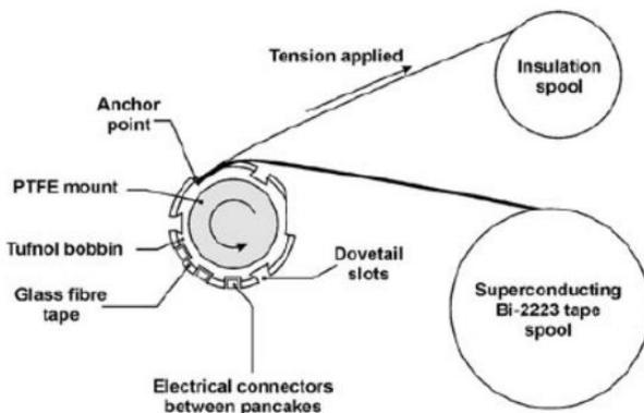
The experimental arrangement for winding the tape and insulation onto the Tufnol bobbin
