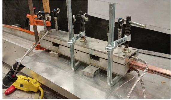
Fig. 4. Aluminum splicing fixture.
