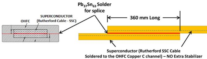
Fig. 3. Typical layout of the test splice for joint resistance evaluation (without any additional copper stabilizer employed in the system).
