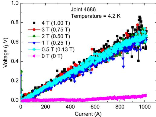
Fig. 8.  $V-I$  data at different magnetic fields for the soldered joint of sample DR4686 at 4.2 K. The two magnetic field values shown are those at the field center and at the top of the joint (in brackets), which was about 150 mm away from the field center. A linear fit to the high-field data, where the solder is normal, gives a resistance of 0.7 n $\Omega$ .
