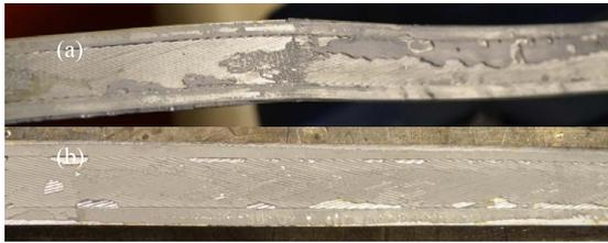
Fig. 5. Conductor after being peeled apart during early splice tests. (a) Large areas that did not adhere uniformly. (b) Change in fixture, flux, and technique resulted in a much more uniform bond between the pieces.
