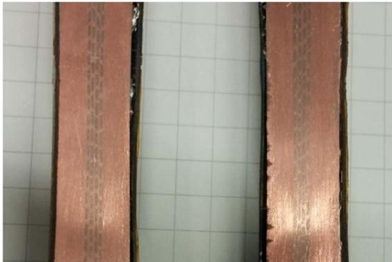
Fig. 6. Splice mock-up end-on view of the sectioned splice cut lengthwise, showing void-free construction. NbTi strands and solder can be seen in the copper matrix. Outer wrap is polyimide film and epoxy.
