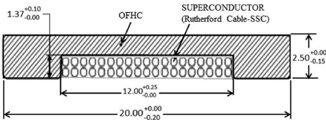
Fig. 2. Torus conductor: SSC outer cable soldered into copper channel (dimensions in millimeters).
