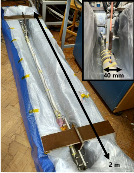
Fig. 2: One of the two Durham set-ups. It includes an open-bucket Dewar and the use of non-magnetic (and non-metallic) materials - a polythene liner and Tufnol cable supports.
