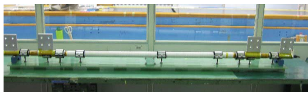
Fig. 1. Measured sample cable. The silver part in the central area is the outer shield conductor. Four copper plates at the both ends are attached to the inner core and to the shield layer.
