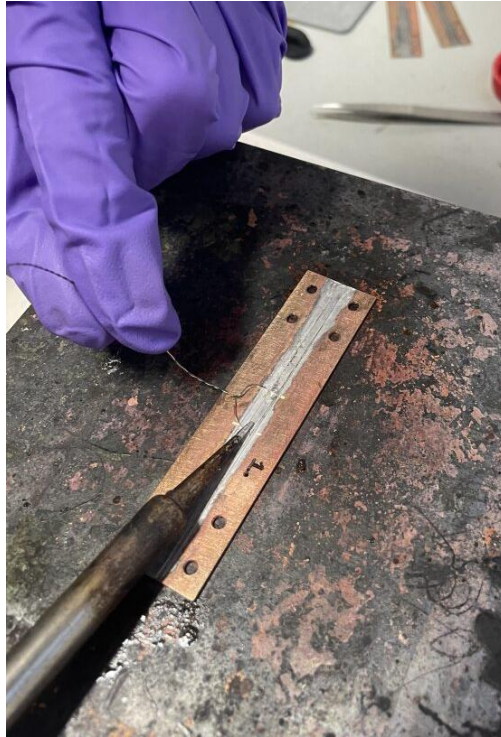
Fig. 6: Soldering the voltage taps.
