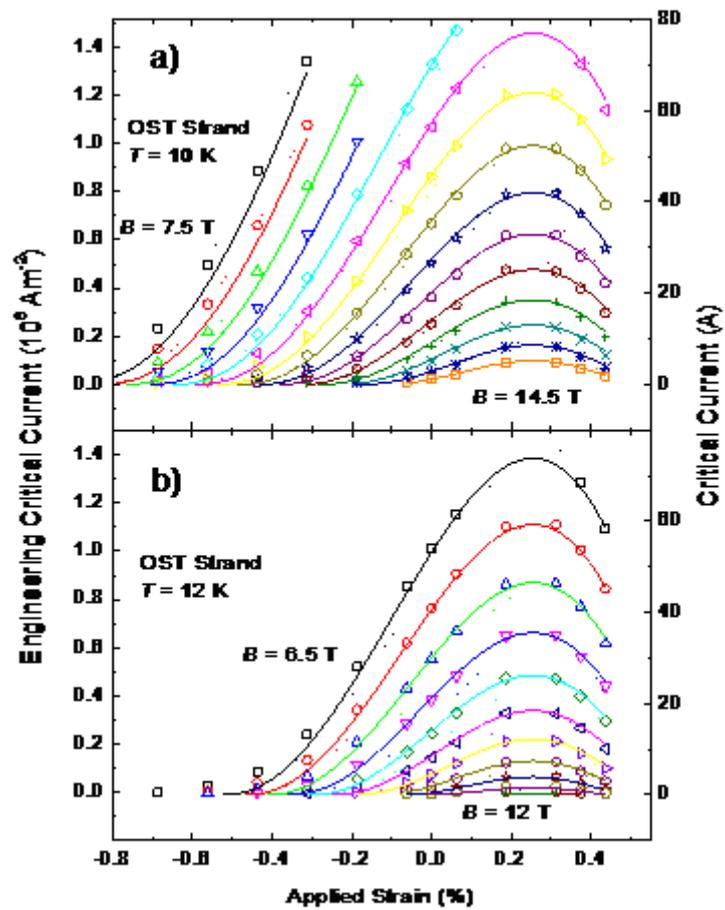
**Fig. 4.** Engineering critical current density (and critical current) of OST strand as a function of applied strain in magnetic fields (a) from 7.5 to 14.5 T at 10 K, and (b) from 6.5 to 12 T at 12 K. The increment of the magnetic fields is 0.5 T. The solid lines are provided from fitting the 9 free-parameter Durham scaling law. The dotted lines are provided by the ITER scaling law.
