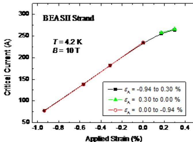
**Fig. 13:** The critical current as a function of applied strain at 10 T and at  $T = 4.2$  K, for the BEASII strand. The lines are guides to the eye.
