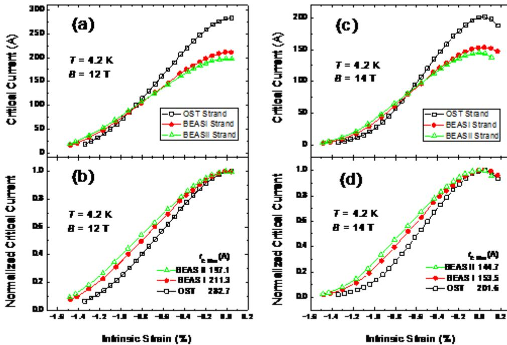
**Fig. 16:** Critical current and normalized critical current as functions of intrinsic strain at  $T = 4.2 \text{ K}$  and at magnetic fields equal 12 and 14 T for the three strands measured in this report. The lines are guides to the eye.
