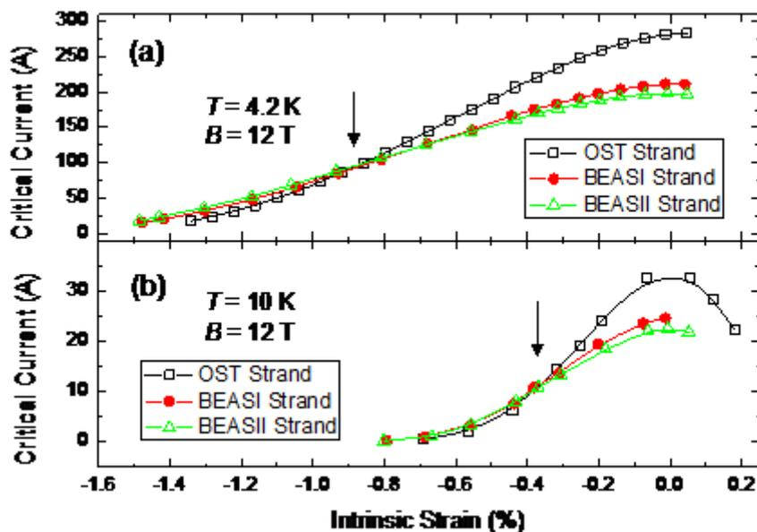
**Figure 18:** Intrinsic strain dependence of critical current ( $I_C$ ) at 12 T and at (a) 4.2 K and (b) 10 K for all three strands measured. At a fixed temperature  $I_C$  of all strands meet at one intrinsic strain as indicated by arrows in the figure.
