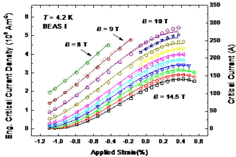
**Figure 8.** Engineering critical current density (and critical current) as a function of applied strain at 4.2 K and magnetic fields between 8 and 14.5 T for the BEASI strand. The solid lines are provided by the Durham scaling law<sup>6</sup> using 9 free parameters listed in table IV. The dotted lines are provided by the ITER scaling law<sup>7</sup> (parameters in table V)
