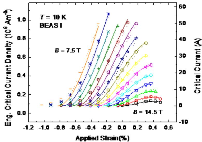
**Figure 9.** Engineering critical current density (and critical current) as a function of applied strain at 10 K and magnetic fields between 7.5 and 14.5 T for the BEASI strand. The solid lines are provided by the Durham scaling law<sup>6</sup> using 9 free parameters listed in table IV. The dotted lines are provided by the ITER scaling law<sup>7</sup> (parameters in table V).
