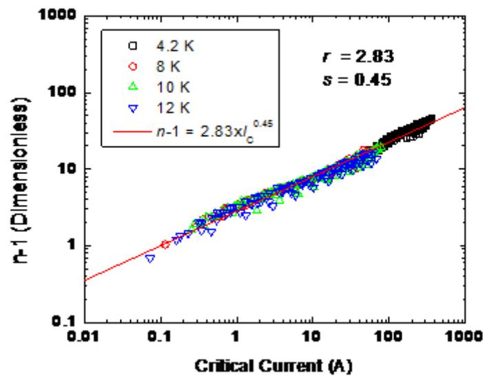
**Fig. 7:** The  $n$ -value obtained from fitting the experimental data to the equation  $E = \alpha J^n$  over the range from 10 to 100  $\mu\text{Vm}^{-1}$ . Data are shown for the OST strand plotted as  $n-1$  as a function of critical current at  $T = 4.2 \text{ K}$ , 8 K, 10 K and 12 K in different fields. The line shows a fit to all the data using equation (9) where  $r = 2.83$  and  $s = 0.45$ .
