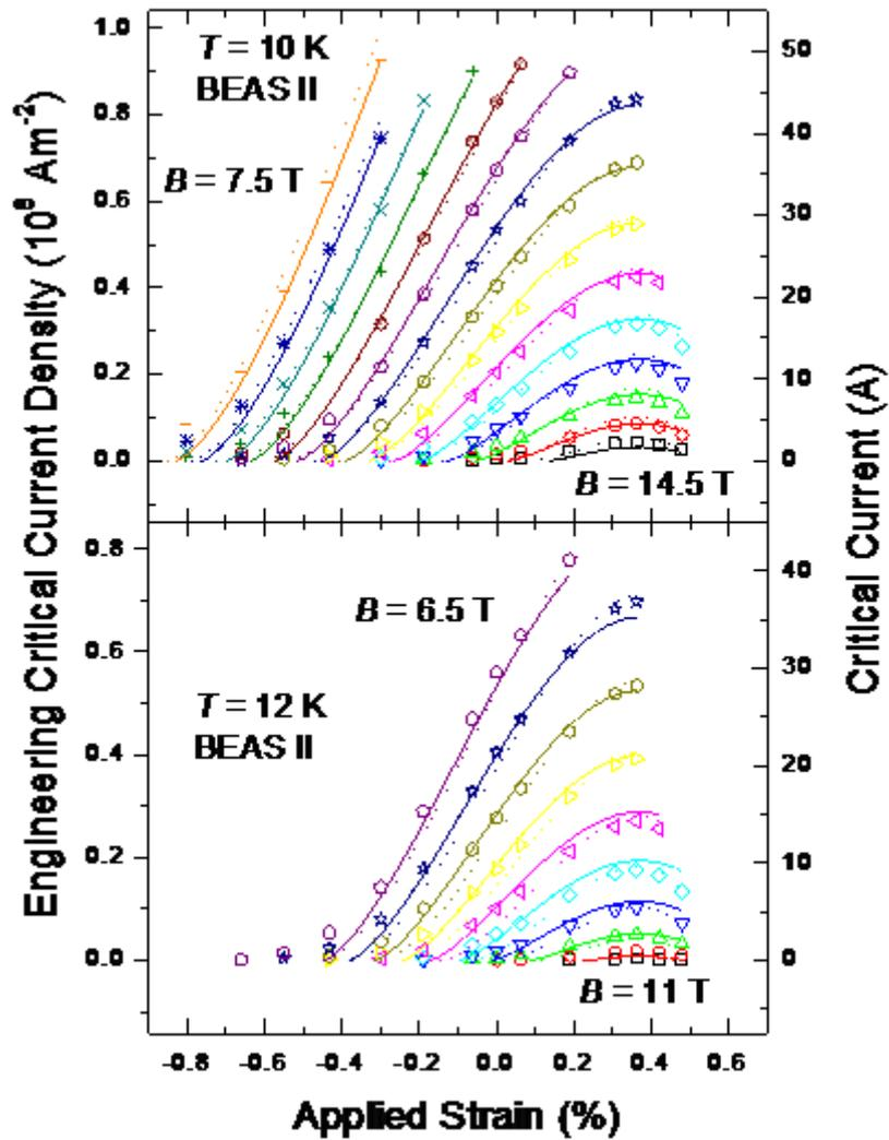
**Figure 11.** Engineering critical current density (and critical current) of BEASII strand as a function of applied strain at (a) 10 K in magnetic fields from 7.5 to 14.5 T in increments of 0.5 T and at (b) 12 K in fields from 6.5 to 11 T in increments of 0.5 T. The solid lines are provided by the Durham scaling law<sup>6</sup> using 9 free parameters listed in table VI. The dotted lines are provided by the ITER scaling law<sup>7</sup> (parameters in table VII).
