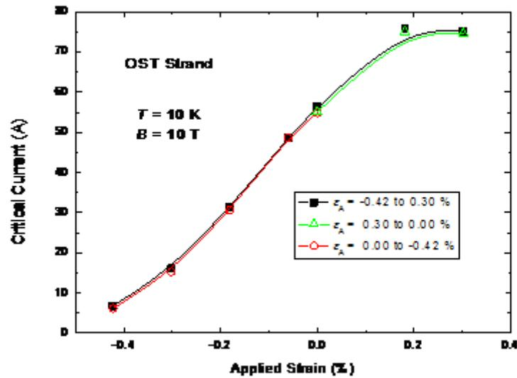
**Fig. 5:** The critical current as a function of applied strain at 10 T and at  $T = 10$  K, for the OST strand. The lines are guides to the eye.
