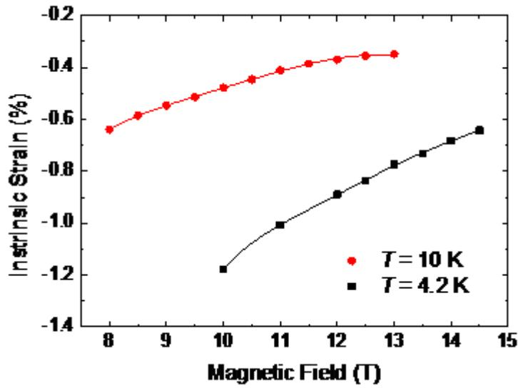
**Figure 19:** Pivot points of the strands at 4.2 K and 10 K. The lines are guides to the eye.
