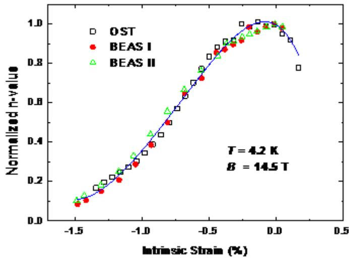
**Fig. 20:** Normalized  $n$ -values as a function of intrinsic strain for the three strands measured in this report. The line is guide to the eye.
