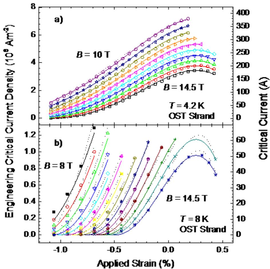
**Fig. 3.** Engineering critical current density (and critical current) of OST strand as a function of applied strain at (a) 4.2 K in magnetic fields from 10 to 14.5 T in increments of 0.5 T and at (b) 8 K in fields from 8 to 14.5 T in increments of 0.5 T. The solid lines are provided by the Durham scaling law<sup>6</sup> using the 9 free parameters listed in table II. The dotted lines are provided by the ITER scaling law<sup>7</sup> (parameters in table III).
