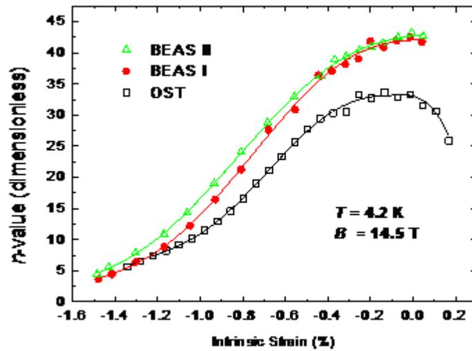
**Fig. 6:**  $n$ -value as a function of intrinsic strain for OST strand compared with other BEAS strands. Lines are guides to the eyes.
