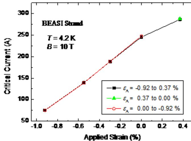
**Fig. 12:** The critical current as a function of applied strain at 10 T and at  $T = 4.2$  K, for the BEASI strand. The lines are guides to the eye.
