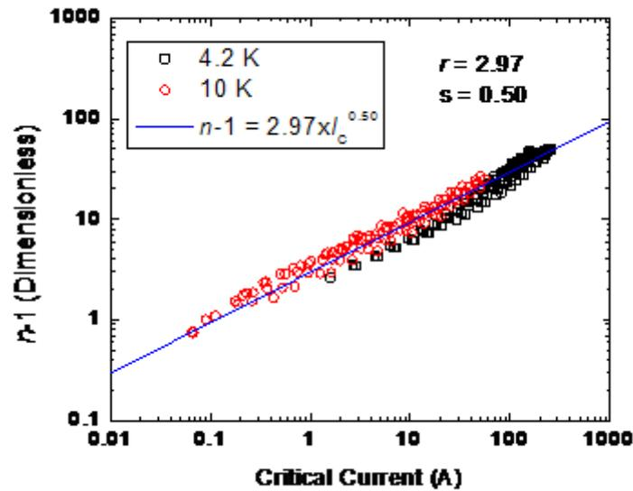
**Fig. 14:** The  $n$ -value obtained from fitting the experimental data to the equation  $E = \alpha J^n$  over the range from 10 to 100  $\mu\text{Vm}^{-1}$ . Data are shown for the BEASI strand plotted as  $n-1$  as a function of critical current at  $T = 4.2$  K and 10 K in different fields. The line shows a fit to all the data using equation (9) where  $r = 2.97$  and  $s = 0.50$ .
