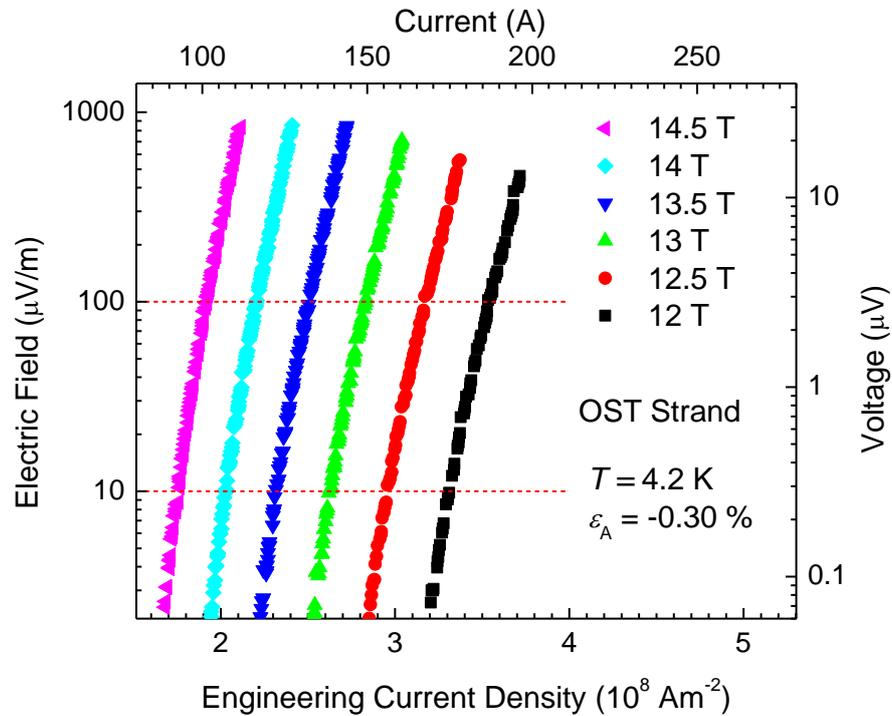
**Fig. 2.** Log-log plot of electric field versus current (and voltage versus current) for the OST strand at 4.2 K, with  $\epsilon_A = -0.30\%$  in magnetic fields between 12 T and 14.5 T in increments of 0.5 T.
