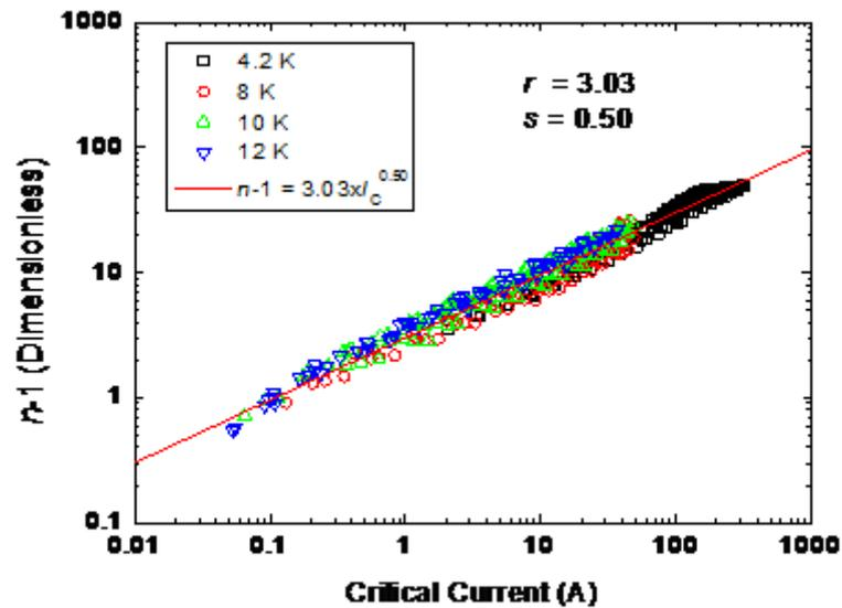
**Fig. 15:** The  $n$ -value obtained from fitting the experimental data to the equation  $E = \alpha J^n$  over the range from 10 to 100  $\mu\text{Vm}^{-1}$ . Data are shown for the BEASII strand by plotting  $n-1$  as a function of critical current at  $T = 4.2$  K, 8 K, 10 K and 12 K in different fields. The line show a fit made using equation (9), where  $r = 3.03$  and  $s = 0.50$ .
