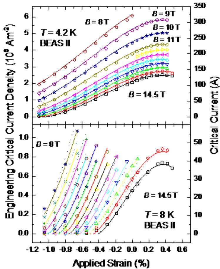
**Figure 10.** Engineering critical current density (and critical current) of BEASII strand as a function of applied strain at (a) 4.2 K in magnetic fields from 8 to 14.5 T and at (b) 8 K in fields from 8 to 14.5 T in increments of 0.5 T. The solid lines are provided by the Durham scaling law<sup>6</sup> using 9 free parameters listed in table VI. The dotted lines are provided by the ITER scaling law<sup>7</sup> (parameters in table VII).
