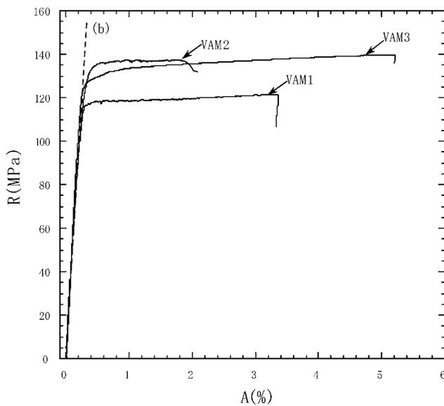
**Figure 1.** Typical  $R$ – $A$  curve for three different tapes, VAM1, VAM2 and VAM3.
