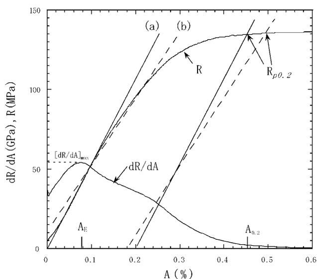
**Figure 2.** Extension dependence of  $R$  and  $dR/dA$  for tape VAM2. Here  $A_E$  and  $A_{0.2}$  are the extensions corresponding to  $[dR/dA]_{\max}$  and  $R_{p0.2}$ , respectively.
