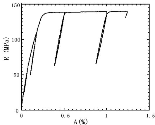
**Figure 3.** Unloading/reloading test, where the unloading took place at 0.05, 0.15, 0.5 and 1% of percentage extension for tape VAM2.
