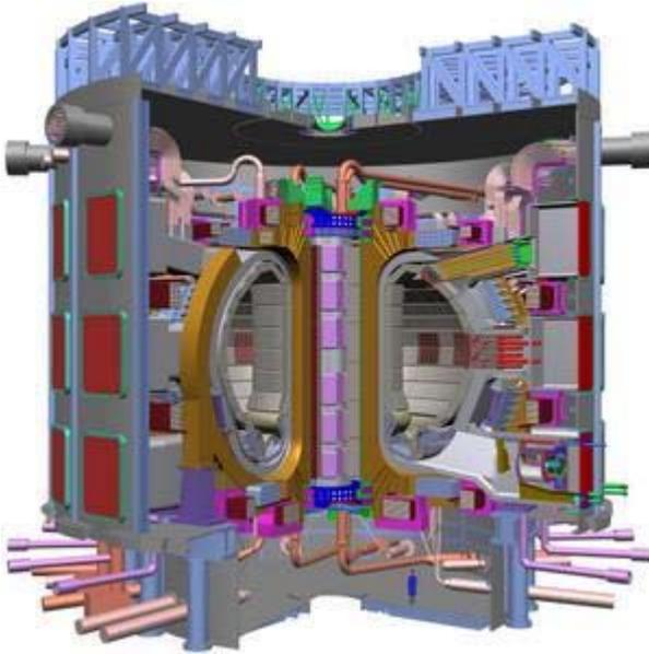
Cutaway of the ITER tokamak.
