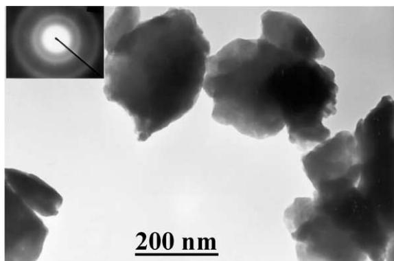
Fig. 4. Bright-field TEM micrograph and electron diffraction pattern of the PMS sample ball-milled for 200 h.
