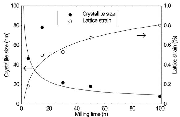
Fig. 3. Variation of crystallite size and lattice strain with milling time derived from the XRD analysis.
