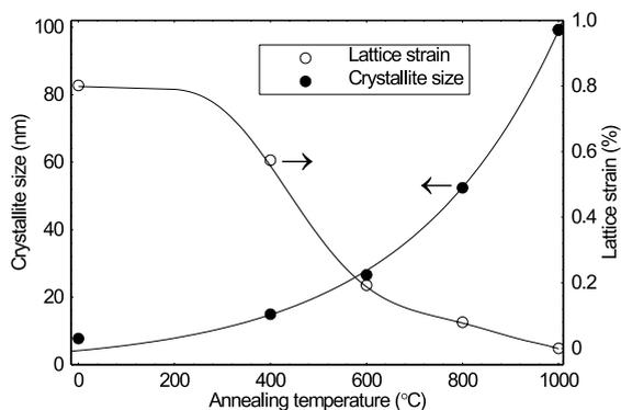
Fig. 6. Variation of crystallite size and lattice strain with annealing temperature derived from the XRD analysis for 100 h ball-milled sample. Lines shown are a guide to the eye.
