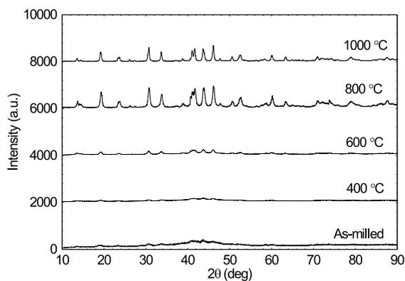
Fig. 5. XRD patterns of PMS samples annealed at different temperatures. The sample was ball-milled for 100 h before annealing.
