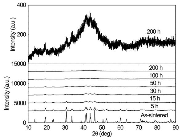
Fig. 2. XRD patterns of PMS samples ball-milled for different times.
