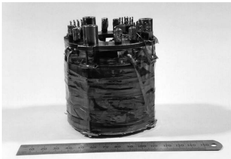
Figure 5. Photo of Bi-2223 magnet.
